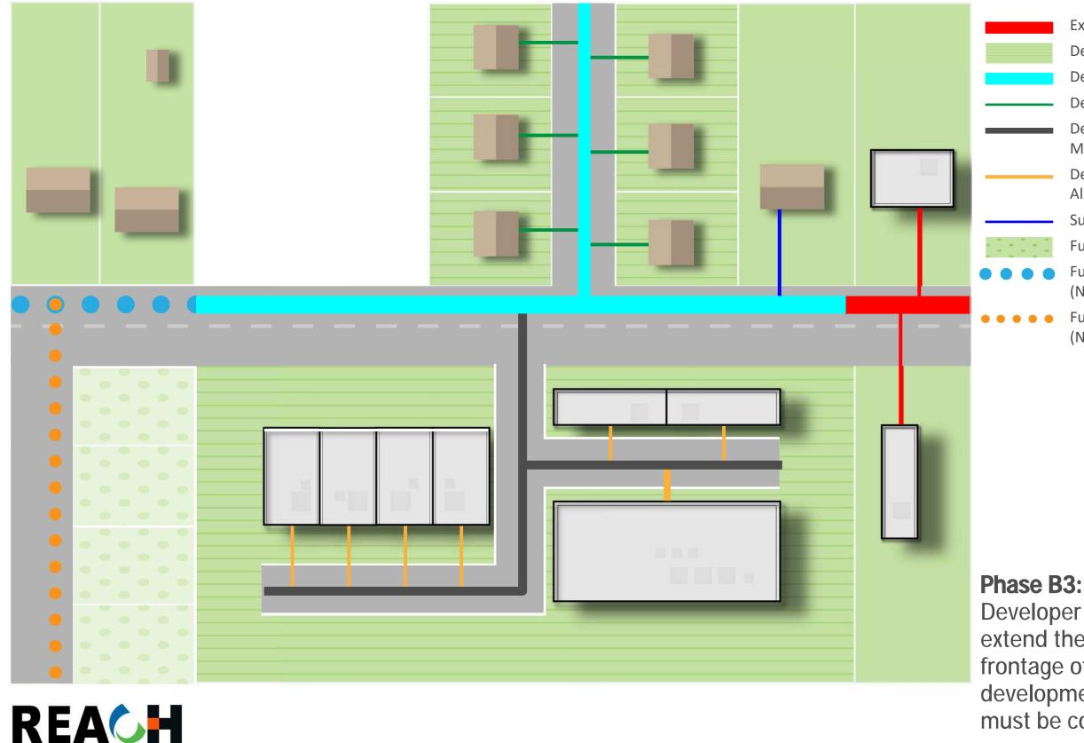
**Existing Mains and Service Lines** Developer A Project Area **Developer A Public Main Extension** Developer A Direct Connect - Revenue Allowance Developer A Commercial Service Line/Private Main Developer A Indirect Connect - Revenue Allowance Subsequent Connector - Owed to Developer A Future Developer B Project Area Future Developer B Public Offsite Main Extension (Nothing Owed to Developer A or C)
