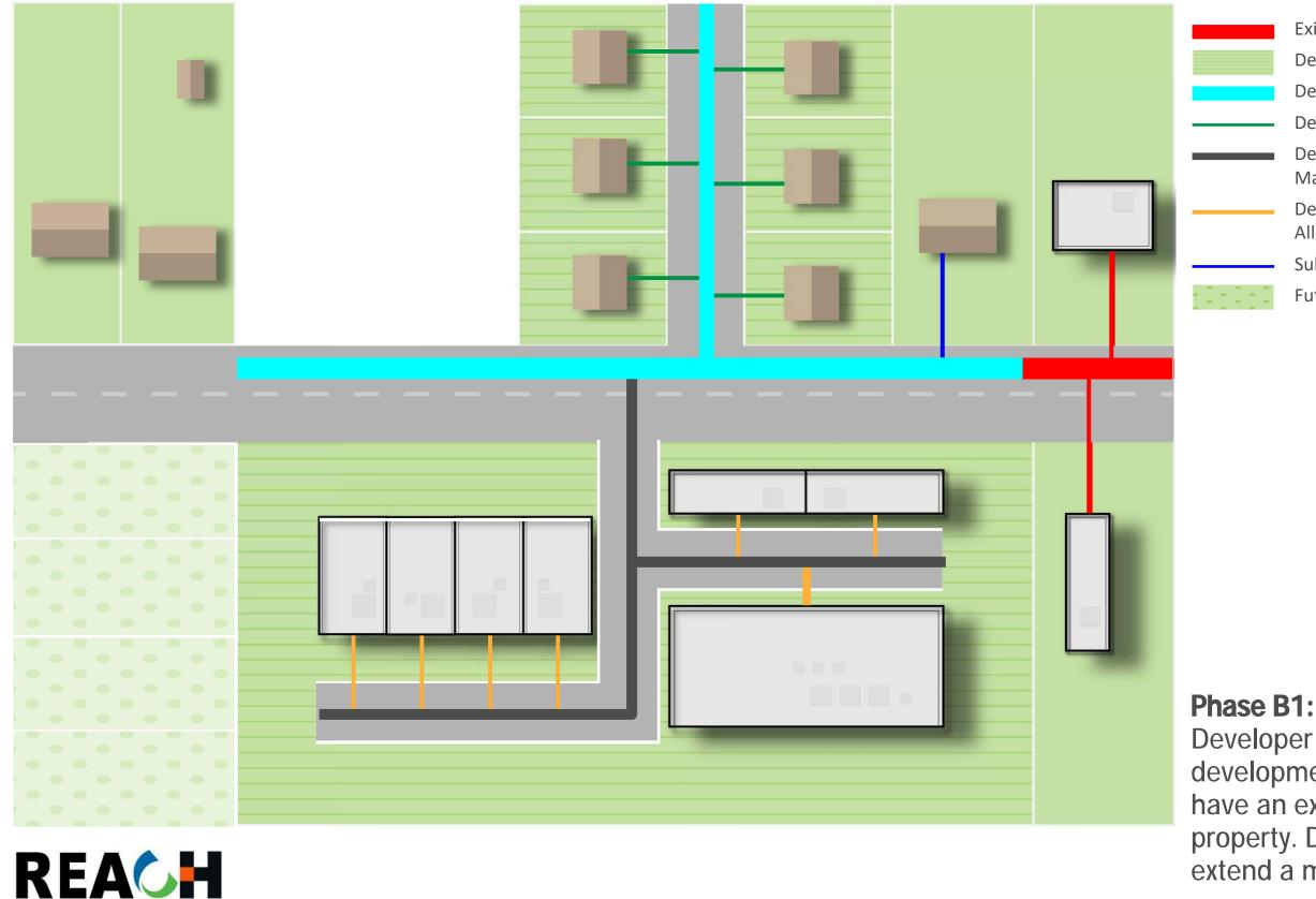
**Existing Mains and Service Lines** Developer A Project Area **Developer A Public Main Extension** Developer A Direct Connect - Revenue Allowance **Developer A Commercial Service Line/Private** Main Developer A Indirect Connect - Revenue Allowance Subsequent Connector - Owed to Developer A Future Developer B Project Area
