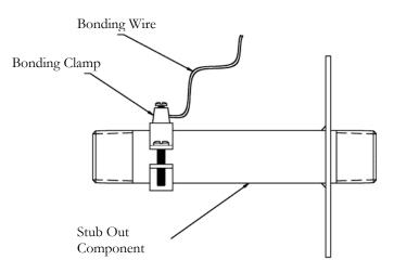
Figure 2 Bonding Clamp on Steel Pipe Segment (Remove any paint or coating on pipe surface beneath clamp location)
