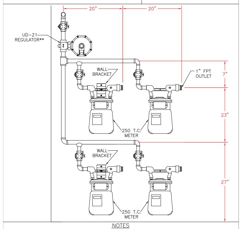
PREFABRICATED METER ASSEMBLY SPLIT FOR FOUR METERS
